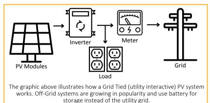
your solar PV array also shuts down. This is done to prevent injury to utility line workers that may be performing repairs. This type of system design also allows for net metering.
